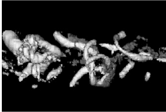
Figure 12. NM calculation at t = 60 . Tridimensional view of the pressure (bright surfaces) and the density (dark surfaces) fields. Pressure surface satisfies the relation P_{\text{iso}} = P_1 + 0.2 \times (P_{\text{min}} - P_1) , where P_1 and P_{\text{min}} denote the initial uniform pressure value and the minimum pressure value at the time considered, respectively. Density surface corresponds to the minimum density value at the time considered.
